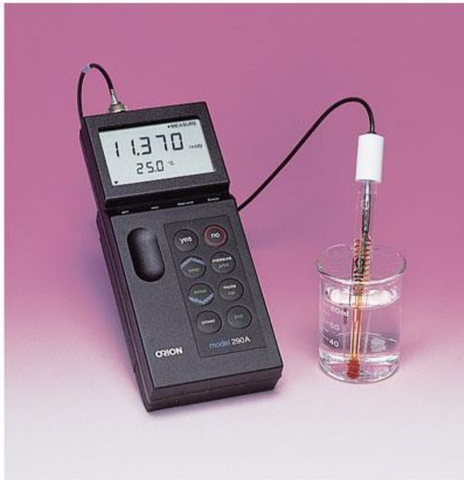
Figure 7.4: (a) Measuring the pH of vinegar. (b) Measuring the pH of aqueous ammonia.
